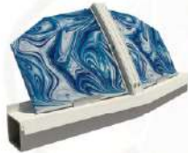
STAINED GLASS LAYER ON TOP OF 3MM POLY-CARBONATE SHEET AS ADDITIONAL TO THE SKYLIGHT DESIGN
