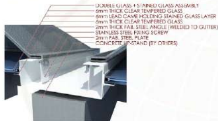
SEC. DET. "T1" A-12 DIM. IN mm NTS
