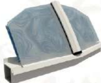
4mm THICK POLY-CARBONATE SHEET FIXED BY ALUMINUM COVER PROFILE AS OUTER LAYER PROTECTION
