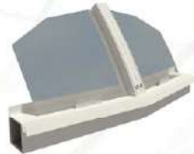
3mm THICK POLY-CARBONATE SHEET PLACED AS INNER LAYER PROTECTION
