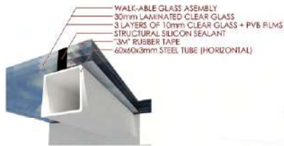
1D SECTION - "1D" SCALE: 1:5
