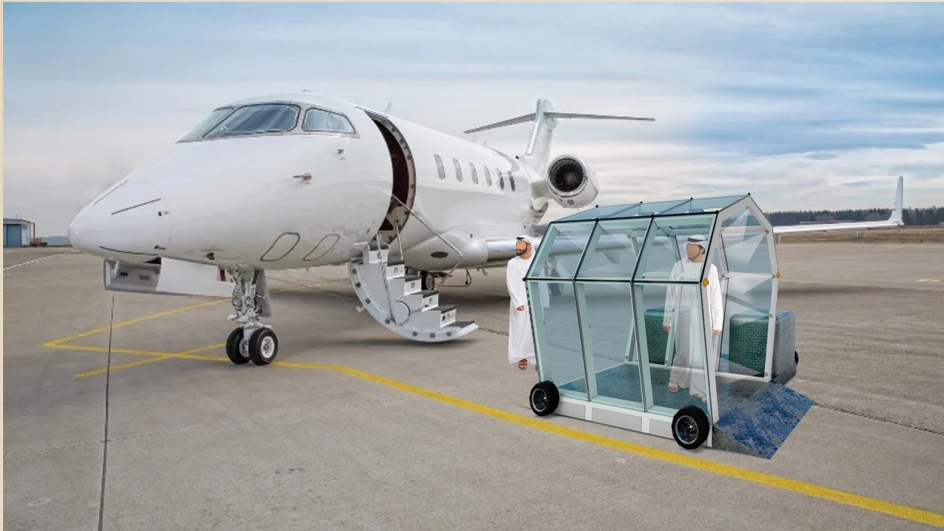
Airport sterilization lane equipped with mobility tires, generator, sterilizer tank and hook
