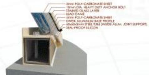
3mm THICK FABRICATED ALUMINUM ANGLE TIED ON TOP OF BASE PROFILE
